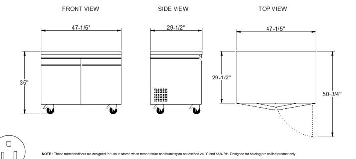
NOTE : These merchandisers are designed for use in stores when temperature and humidity do not exceed 24 °C and 55% RH. Designed for holding pre-chilled product only.
