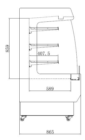
NOTE: These merchandisers are designed for use in stores when temperature and humidity de not exceed 24 °C and 55% RN. Designed for holding pre-chilled product only.
